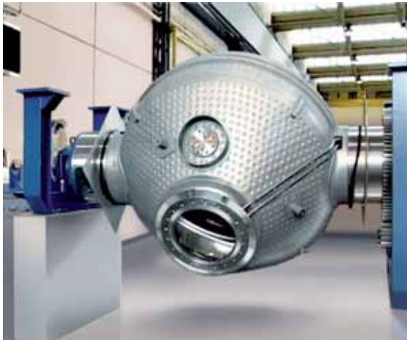
Double Conical Dryer SR 1000: Stainless steel design with ruffled cover
