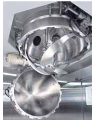
Rosenmund Spherical Dryer with top drive 1000 l
