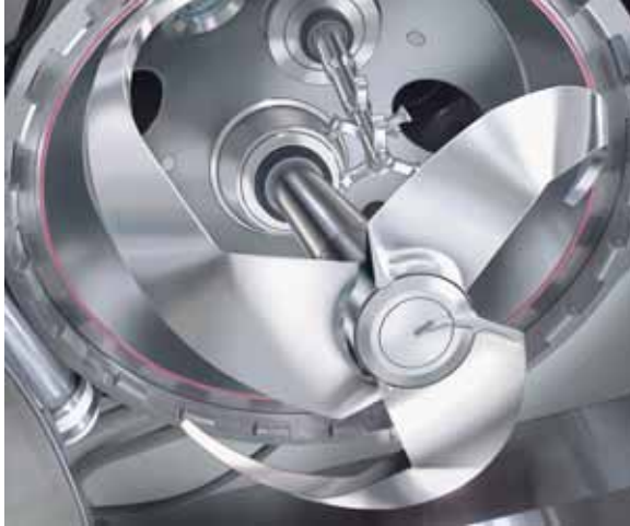
Rosenmund Spherical Dryer with top drive 100 l
