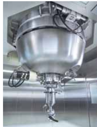
Rosenmund Spherical Dryer with top drive 1000 l
