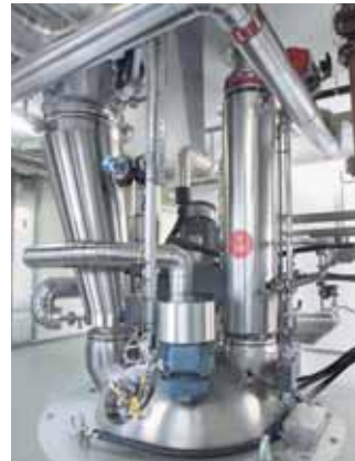
Rosenmund Spherical Dryer with top drive 1000 l
