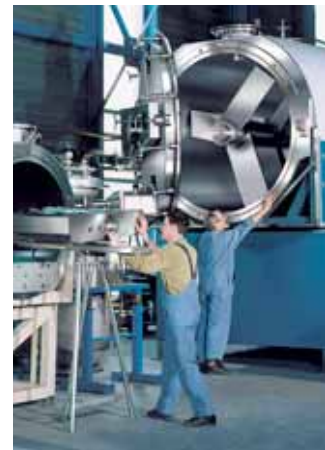
Assembly: Rosenmund Standard Dryer 4000 l
